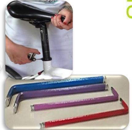
And **lower the seat** so that both feet are flat on the ground. Usually requires a 13mm spanner, Allen key or could be quick release.
